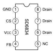
Note: it is □ecommended to connect pin 5 to pin Drain for better heat dissipation.
