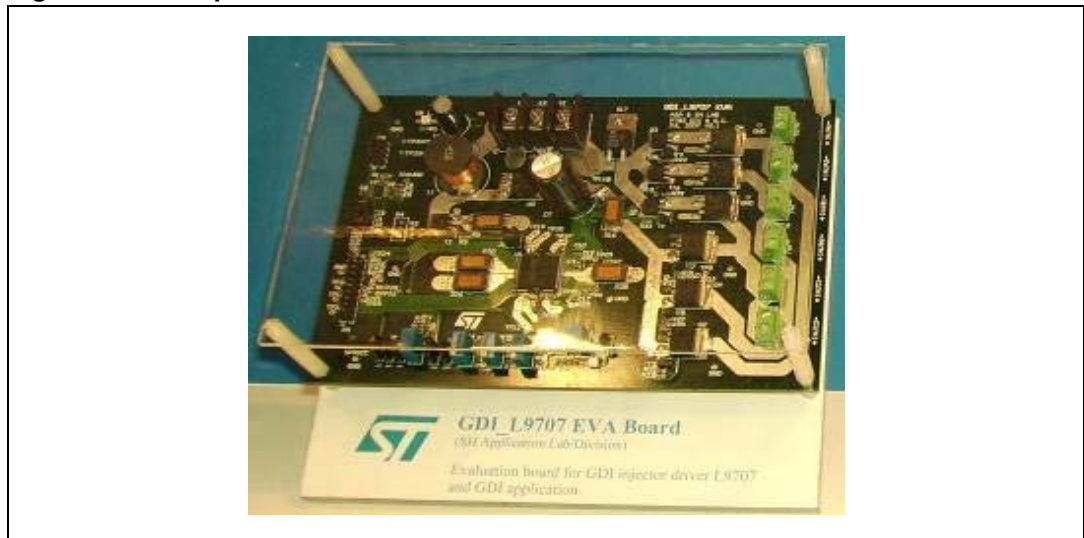
Figure 1. GDI power board based on L9707 and L9777B
