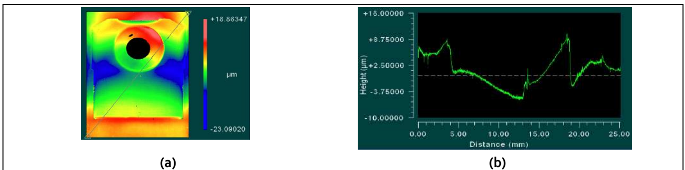
Figure 15 (a) Image and (b) measurement of the planarity of a TO-247-3 along chip's diagonal path
