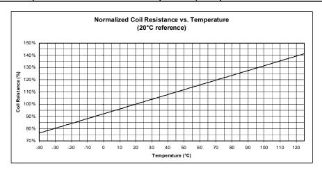
Example: Resistance of  $225\Omega$  coil = 75% of  $225\Omega$  at -40°C, or  $169\Omega$  = 100% of  $225\Omega$  at 20°C, or  $225\Omega$
