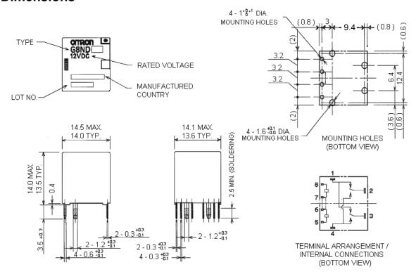
\*\*Note: G8ND-27 R types have 0.7mm (not 0.4mm) standoffs for pin in paste process, to make the effective terminal length 3.2+0.3mm (not 3.5+0.3mm), and the height from the bottom of the standoffs to the top of the case 14.3mm MAX, 13.8mm TYP.
