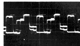
12. Q351 Collector (Y-PCB) 124V, 20 \mu s / Div
